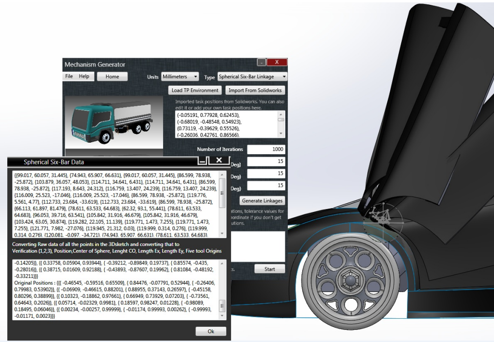
Figure 3.13: Import task position and 3R chain information in MECHGEN
